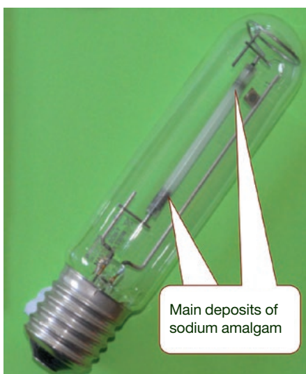
Figure 3: Sodium amalgam deposits in the cooled arc tubes of an HPSV lamp.
