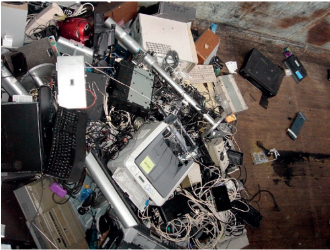
Figure 1: Waste electrical and electronic equipment that was tipped from a great height out of collection boxes into a transport container. It is clear to see that waste electrical and electronic equipment splits open and LIB's can be ejected and damaged in the process.
