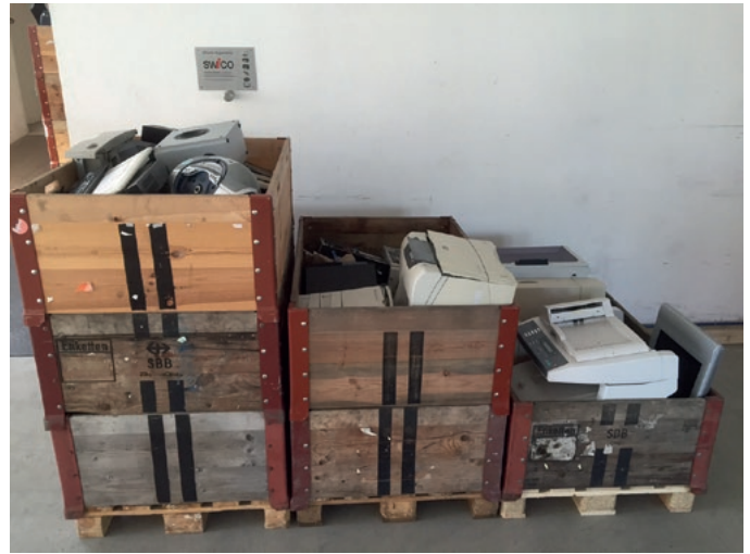
Figure 2: SBB wooden pallets with wooden boxes at a Swico collection point. In order to prevent damage to waste electrical and electronic equipment, the WEEE must not protrude beyond the maximum three stacked boxes.
