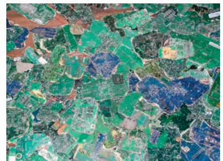
Printed circuit board fractions from manual processing
