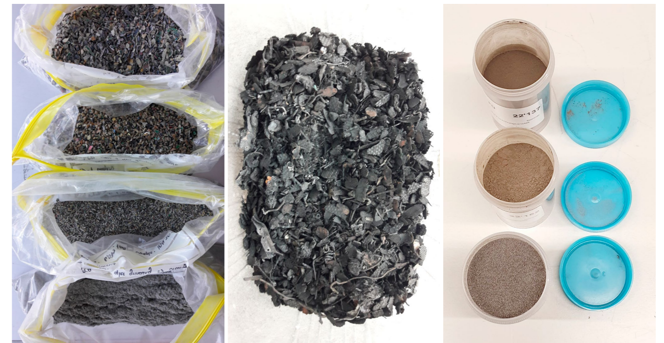
Figure 5: Examples of fractions processed (from left to right): Screen fractions of different grain sizes of ground circuit boards (CB), used to study the distribution of different substances (especially precious metals) in the various matrices; pyrolysed CB fraction, from which all volatile components were removed and separated in solutions and analysed; grinding fractions produced in cryogenic mills (from bottom to top: plastic fraction, wet scrubber sludge, RESH).
