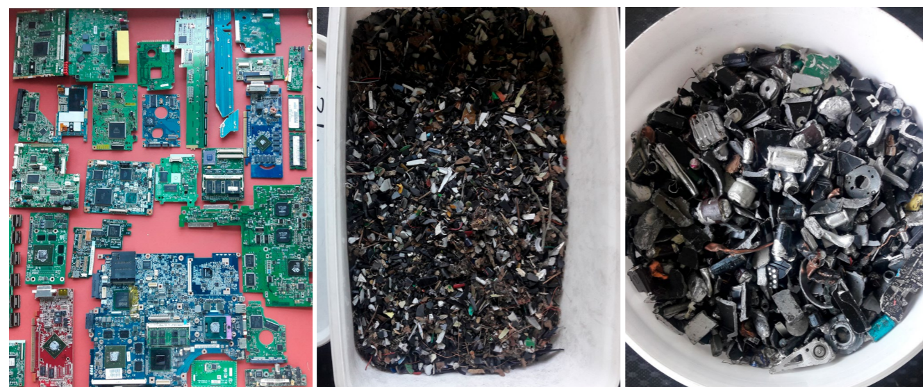
Figure 4: Examples of fractions produced (from left to right): Class 1 circuit boards obtained from the fine dismantling of modern electronic equipment; plastic fraction with a high precious metal content (significant fraction of broken circuit boards) screened out in batch tests; aluminium fraction obtained in batch tests by means of an eddy current separator. A number of electrolyte capacitors can be seen which, although slightly damaged during processing, were almost completely separated in this fraction.
