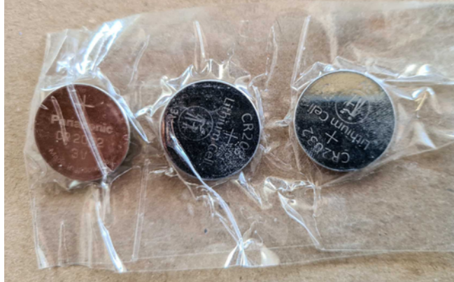
Masked off lithium button cells prevent short circuits in larger quantities (photo: soRec)
