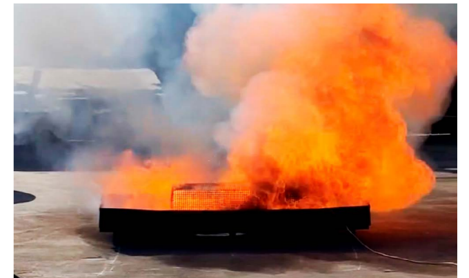
Photo 3: Phase 2 – The battery is on full fire and generates an enormous heat wave.
