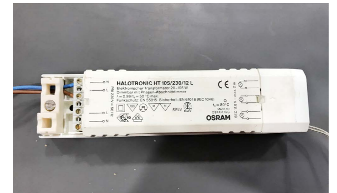
Photo 3: Electronic ballast unit (not suspected of containing PCBs).
