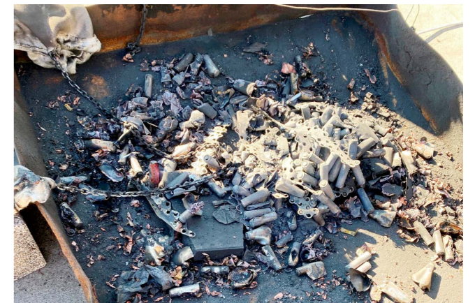
Photo 4: Phase 3 – The residues after completion of the fire test.
