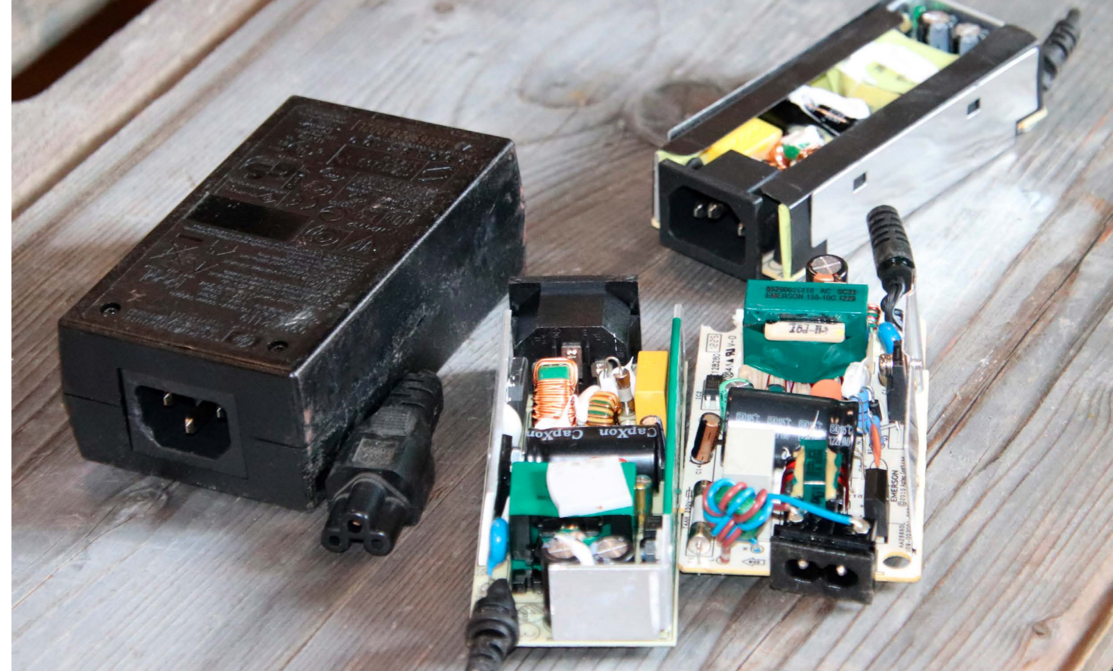
Photo 1: Open power supply units category 2.
