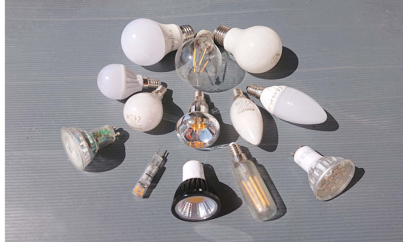
Photo 1: Non-rod-shaped LEDs in 13 different material combinations.
